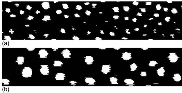
FIG. 15. Cross sections of the lower and upper layers of a QD super lattice under conditions of an initial high-density template. (a) The lower layer has a high density of randomly sized and spaced dots. (b) After 20 layers of growth, the QDs have become more uniform in size and are showing signs of self-organization. This figure indicates that there is no bimodal distribution in the upper layers, therefore indicating that this is not the cause of the double peak observed in the PL measurement.
