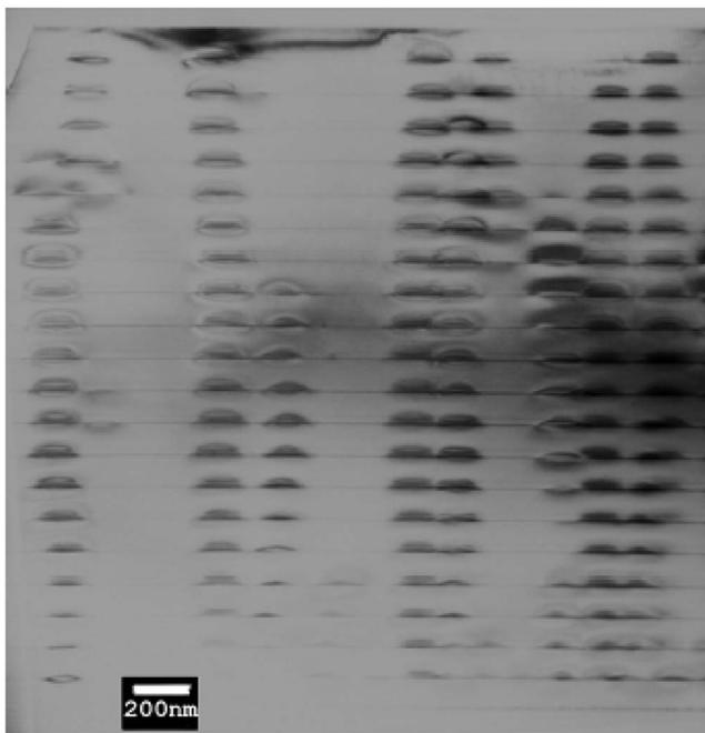
FIG. 8. TEM cross section of a QD superlattice where the template layer has a high density of QDs. As the number of layers progresses, columns realign to distance themselves; when this is not possible, they cease to replicate. Each successive layer of QDs aligns itself to the previous while trying to reorder into a lower energy configuration.
