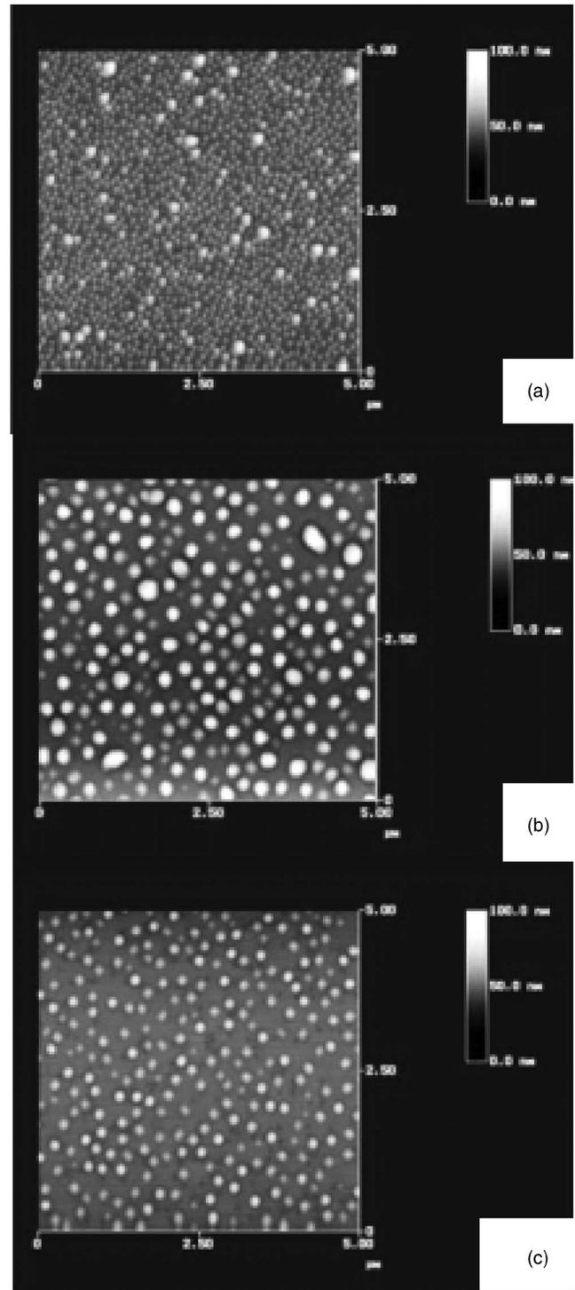
FIG. 2. AFM-generated 2D topology plots of the surface of a sample under conditions of varying growth temperature. The sample grown at 750 °C (c) had a greater degree of size and shape consistency than those grown at 650 °C (a), even after a 30 min annealing cycle (b).
