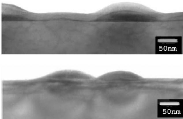
FIG. 4. (Upper panel) Cold capping with Si conformally coats Ge dots. Ge dots (dark domes) retain their shape despite capping with 20 nm of Si at 300 °C. The thin Ge wetting layer is also visible in this image (thin dark line that appears between dots). (Lower panel) Uncapped Ge dots exhibit a domelike shape.
