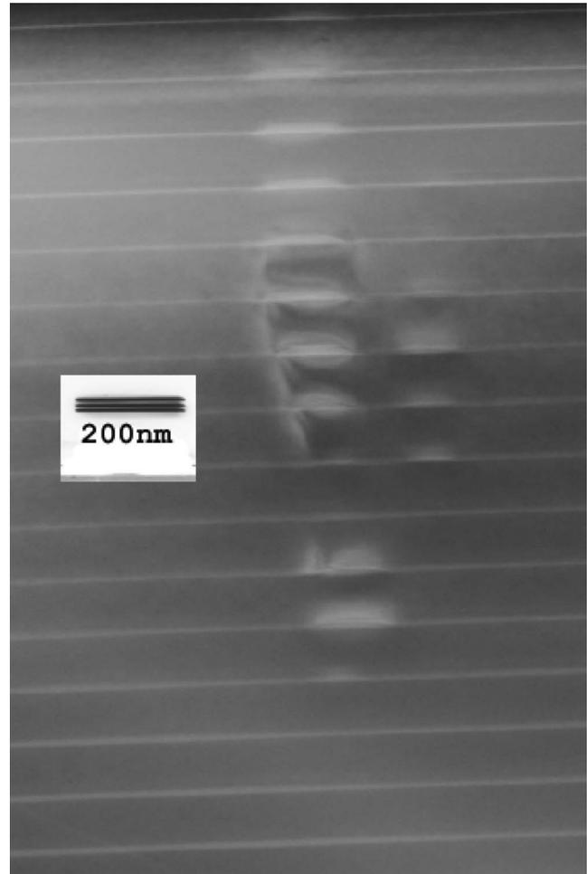
FIG. 9. TEM cross section of a QD superlattice where the template layer has a low density of QDs. As the number of layers progresses, new columns of islands form to lower the surface energy. There was not a QD at this position in the template, but it was energetically favorable for a new column to form. Once a new column is established, each successive layer of QDs aligns to the previous while trying to reorder into a lower energy configuration.
