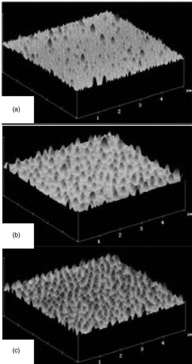
FIG. 1. AFM-generated 3D topology plots of the surface of a sample under conditions of varying growth temperature. The sample grown at 750 °C (c) had a greater degree of size and shape consistency than those grown at 650 °C (a), even after a 30 min annealing cycle (b).
