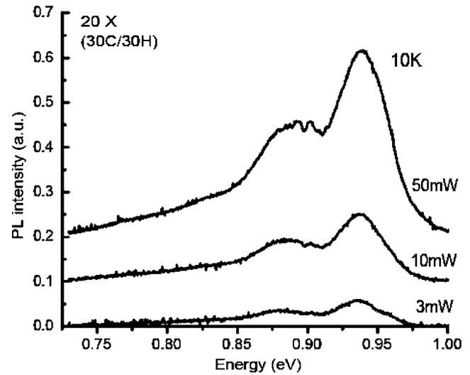
FIG. 13. The temperature dependence PL measurement, on one of the multiple Ge layer samples, illustrates that the lower energy band is a phonon replica of the no-phonon (NP) band and not due to temperature-dependent phenomena. Note that these are two-layer samples. The ratios of NP to phonon replica are independent of temperature, ruling out the explanation as ground and excited states in dots.
