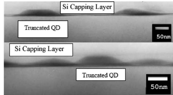
FIG. 5. The tops of taller QDs are more likely to truncate. In the upper TEM image, the QD on the left, which was originally taller than the one on the right, has been truncated at the height of the cold/hot cap interface. The dot on the right is shorter than the interface line, so it maintains its rounded top. In the lower image, the larger QD, which was in the center, became truncated.
