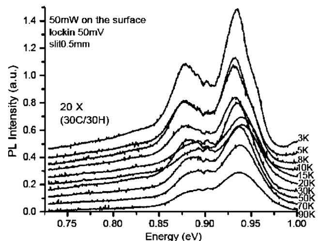
FIG. 14. The pump-power dependence PL measurement, on one of the multiple Ge layer samples, illustrates that the lower energy band is a phonon replica of the no-phonon (NP) band. Note that these are two-layer samples. The ratios of NP to phonon replica are independent of pump power, ruling out the explanation as ground and excited states in dots.
