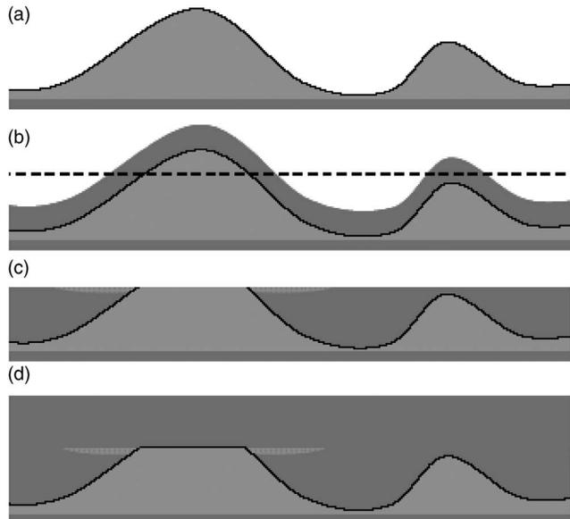
FIG. 7. Truncation model. (a) Two QDs of unequal size. (b) Cold capping of the QDs, which conformally coats them. The dashed line represents the average surface height of the deposited materials. (c) Planarization to the average surface height (dashed line) of the deposited material from annealing after cold capping. QDs taller than this line are truncated. (d) Truncation of QDs at the same spot as shown in (c) resulting from hot capping after cold capping.
