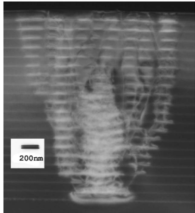
FIG. 16. Dislocations branching out from a large initial dot act as preferential nucleation sites for new layers of QDs, creating a treelike pattern.
