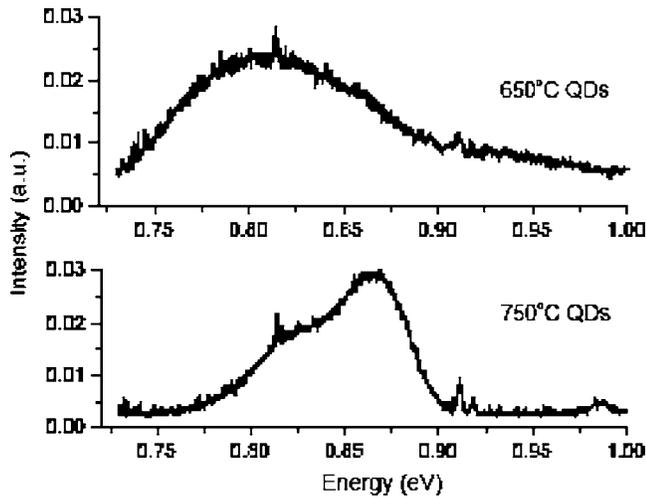
FIG. 3. PL response for similarly prepared QD samples grown at 650 and 750 °C. The sample grown at 750 °C has a greater intensity and larger average energy PL response, indicating that the dots are more uniform in size and distribution than that observed for the samples grown at 650 °C.
