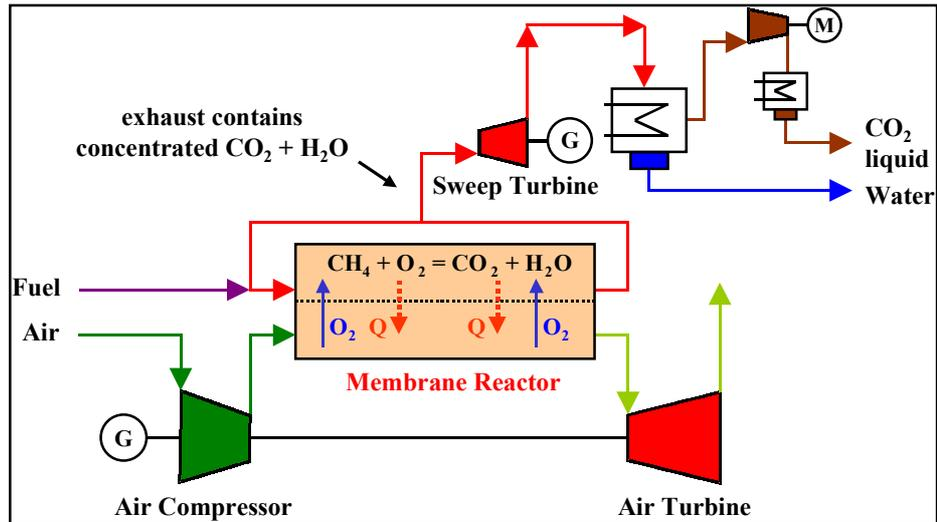
*Figure 5: Zero emissions gas turbine-based power generation concept (including an integrated membrane for production of oxygen)*
