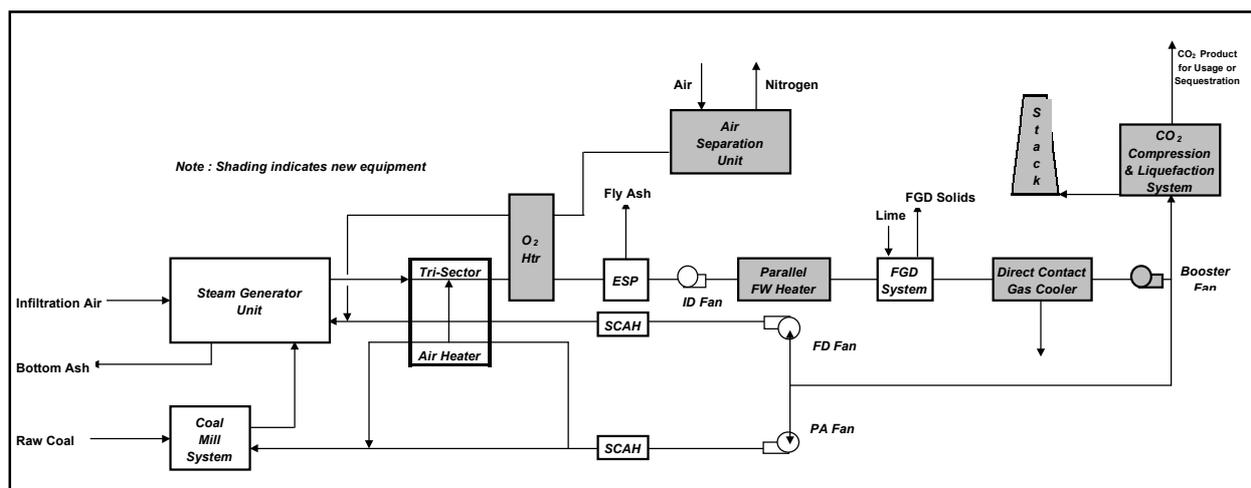
Figure 7: Simplified gas side process flow diagram for CO<sub>2</sub> separation with oxygen firing
