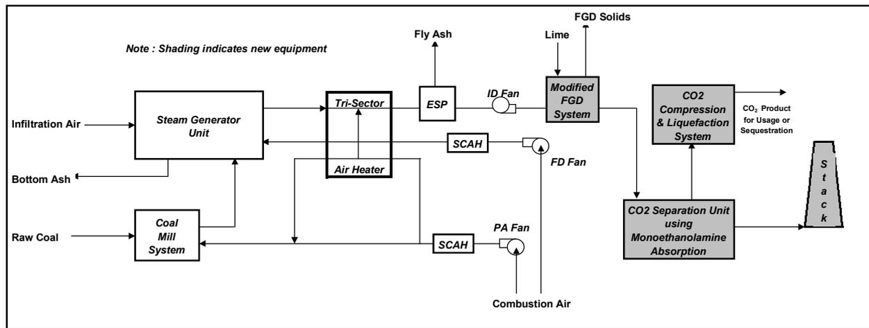
**Figure 8: Simplified gas side process flow diagram for CO<sub>2</sub> separation by MEA absorption**
