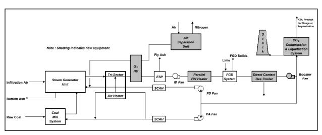
Figure 7: Simplified gas side process flow diagram for CO<sub>2</sub> separation with oxygen firing
