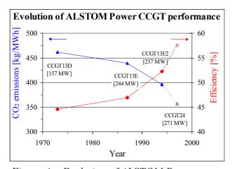
Figure 4a: Evolution of ALSTOM Power CCGT environmental and efficiency performance
