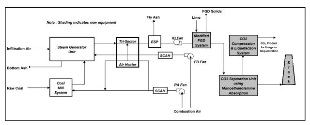
Figure 8: Simplified gas side process flow diagram for CO<sub>2</sub> separation by MEA absorption
