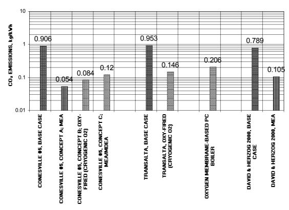
Figure 10: Comparative coal-fired power plant CO<sub>2</sub> emissions
