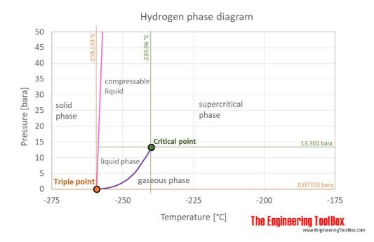
At the **critical point** there is no change of state when pressure is increased or if heat is added.
