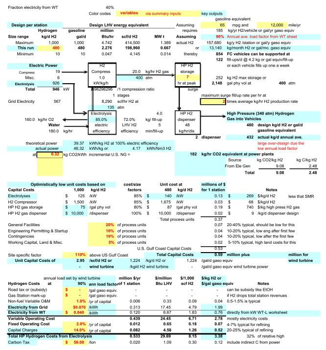
Assume high pressure electrolysis cell with drastically lower capital cost of mass production cost & higher efficiency
