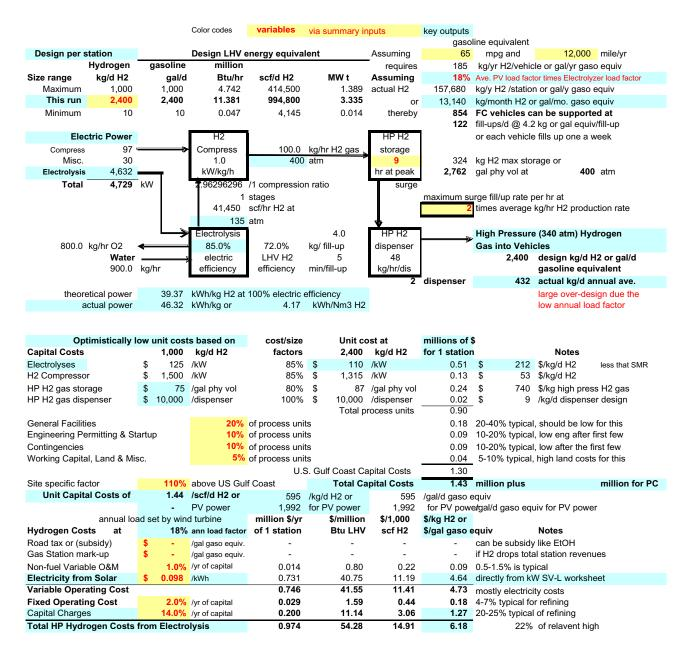
Assume high pressure electrolysis cell with drastically lower capital cost of mass production cost & higher efficiency Assume <a href="mailto:no-re-">no-</a> transmission or distributions cost for the wind turbine power which usually adds \$0.02-.04/kWh Assumed oxygen recovery for by-product sales with large central plant case, but only minor economic impact
