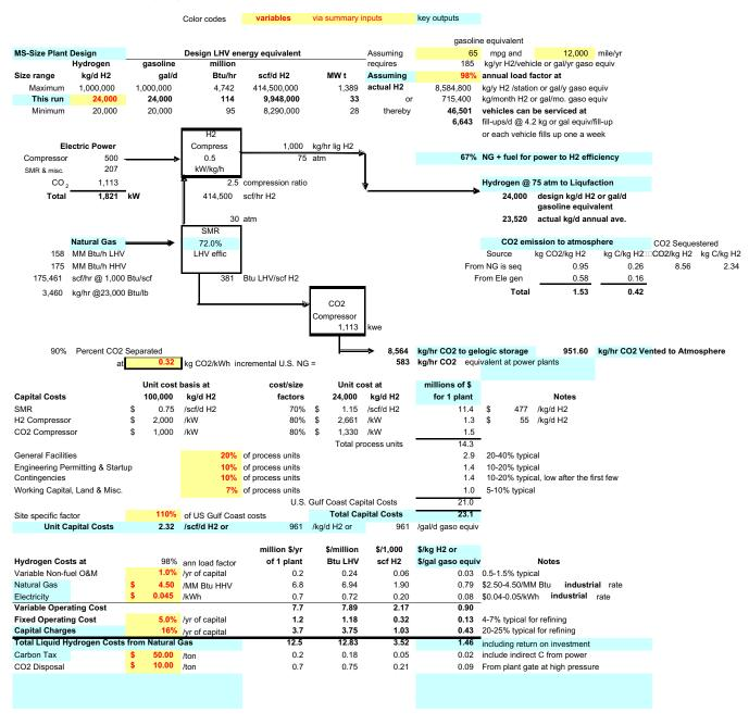
notes: Costs are for production at the plant only and do not include distribution costs. Assume no plant storage and compression of hydrogen to 75 atm for distribution.
