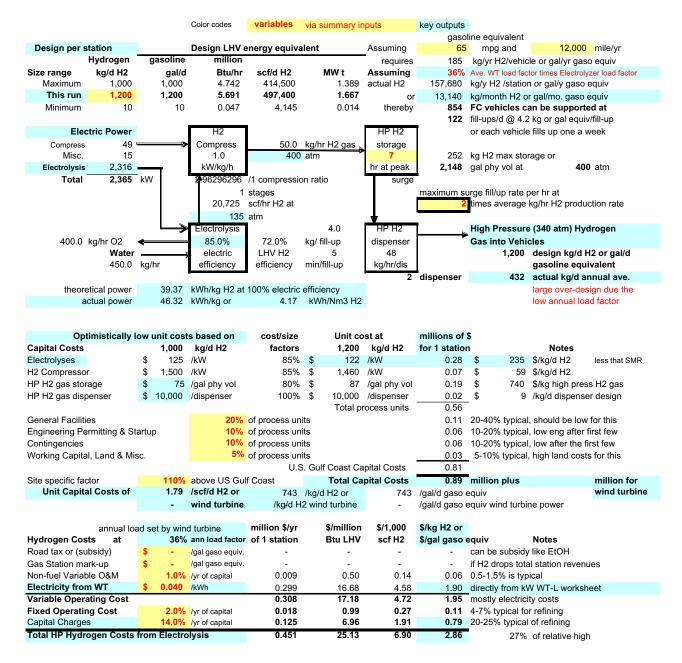
Assume high pressure electrolysis cell with drastically lower capital cost of mass production cost & higher efficiency Assume <u>no</u> transmission or distributions cost for the wind turbine power which usually adds \$0.02-.04/kWh Assumed oxygen recovery for by-product sales with large central plant case, but only minor economic impact
