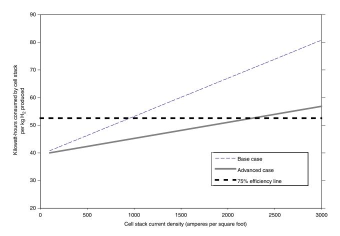
FIGURE G-9 Electrolysis cell stack energy consumption as a function of cell stack current density.
