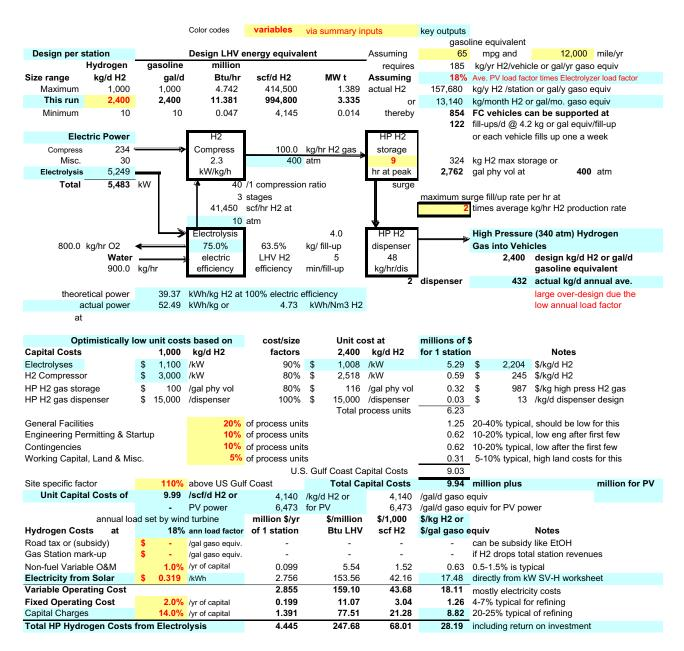
Assume high pressure electrolysis cell with drastically lower capital cost of mass production cost & higher efficiency Assume no transmission or distributions cost for the wind turbine power which usually adds \$0.02-.04/kWh Assumed oxygen recovery for by-product sales with large central plant case, but only minor economic impact
