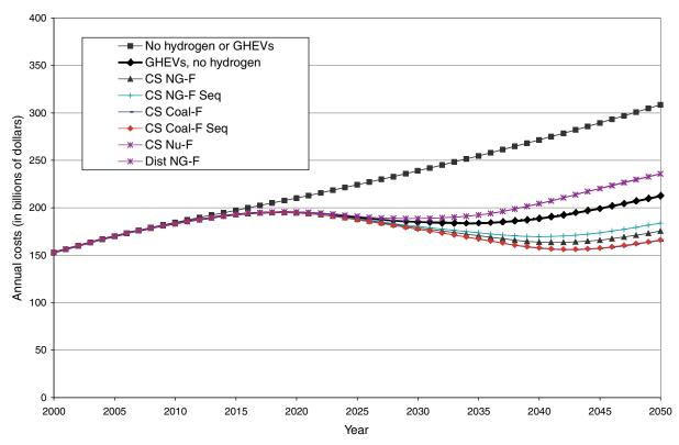
FIGURE 6-22 Estimated total annual fuel costs for light-duty vehicles: possible future hydrogen production technologies (fossil fuels and nuclear energy), 2000–2050. See Table 5-2 in Chapter 5 and discussion in text. NOTE: The cost curve for nuclear thermal energy (CS Nu-F) is obscured by the cost curve for distributed generation from natural gas (Dist NG-F), since these two cost estimates are virtually identical.
