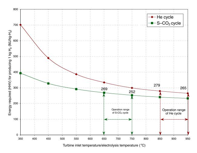
FIGURE G-6 The energy needs for hydrogen production by the gas turbine modular helium reactor (He cycle) high-temperature electrolysis of steam (HTES) and the supercritical  $CO_2$  (S- $CO_2$  cycle) advanced gas-cooled reactor HTES technologies. NOTE: HHV = higher heating value.
