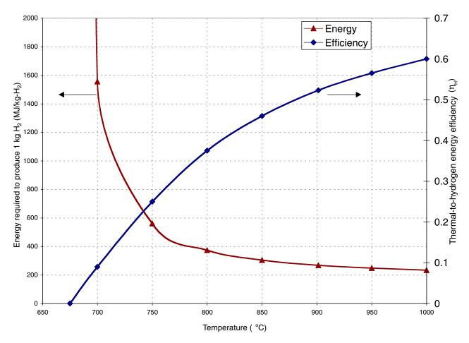
FIGURE G-8 Estimated thermal-to-hydrogen efficiency ( $\eta_H$ ) of the sulfur-iodine (SI) process and thermal energy required to produce a kilogram of hydrogen from the modular high-temperature reactor-SI technology. SOURCE: Brown et al. (2003).
