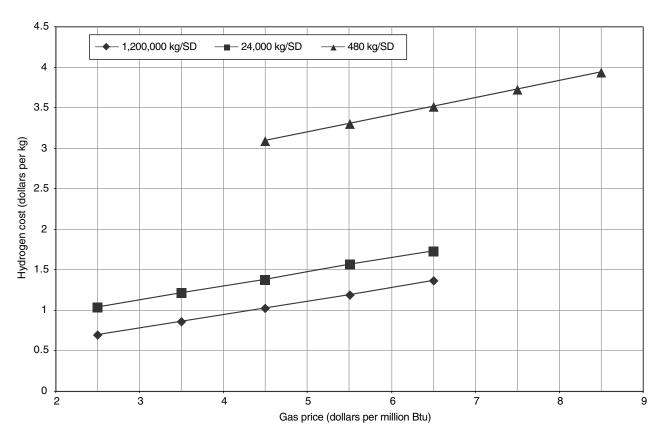
FIGURE G-4 Estimated effects of the price of natural gas on the cost of hydrogen at plants of three sizes using steam methane reforming. Costs based on current technology. NOTE: SD = stream day.
