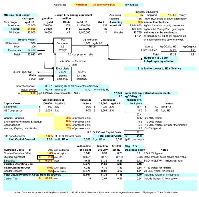
Note: if 12 hr/d at only \$ 0.020 /kWh lower off-peak rate and \$ 0.060 /kWh higher peak rate daily average rate is \$ 0.040 /kWh lift only operated during low off-peak rates times would have low ann load factor & need more H2 storage
