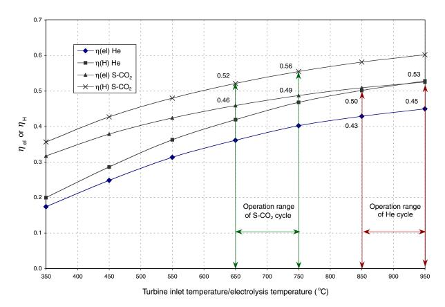
FIGURE G-5 Power cycle net efficiency ( $\eta_{el}$ ) and thermal-to-hydrogen efficiency ( $\eta_{H}$ ) for the gas turbine modular helium reactor (He) high-temperature electrolysis of steam (HTES) and the supercritical  $CO_2$  (S-CO<sub>2</sub>) advanced gas-cooled reactor HTES technologies. SOURCE: Yildiz and Kazimi (2003).
