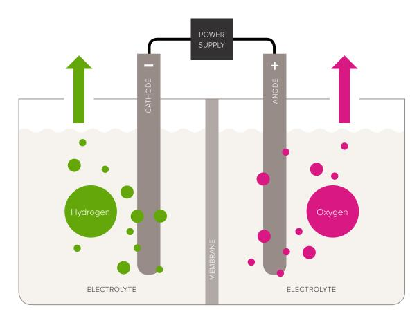
The production of hydrogen and oxygen through electrolysis
