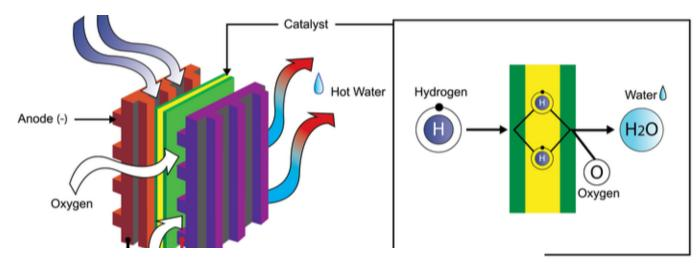
Although less efficient than electric batteries, today's hydrogen fuel cells compare favourably with internal combustion engine technology, which converts fuel into kinetic energy at roughly 25 per cent efficiency. A fuel cell, by contrast, can mix hydrogen with air to produce electricity at up to 60 per cent efficiency.
