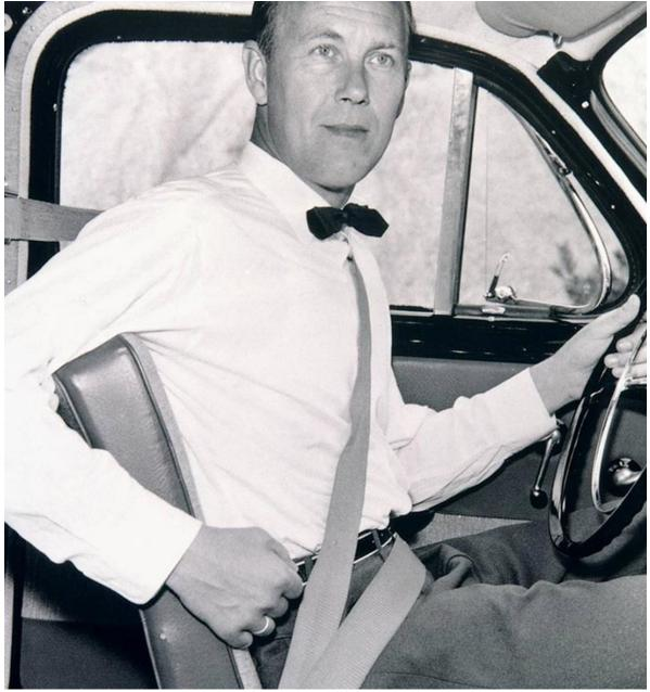
Volvo engineer Nils Bohlin demonstrating the three-point safety belt in 1959. Since then, it's estimated that over one million lives have been saved as a result of Volvo Cars waiving its patent rights. Photo: Volvo Car Corporation.
