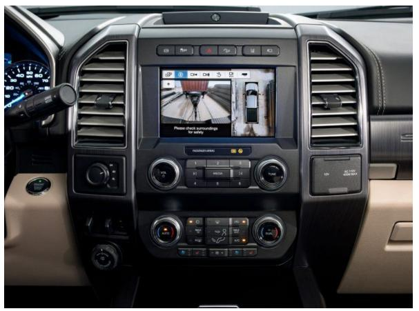
Trailer Reverse Guidance, a new feature for the 2020 Ford Super Duty, shows trailer angle and direction, and provides steering suggestions to assist the driver with backing. The system accommodates all trailer styles, including fifth-wheel and gooseneck applications. Photo: Ford Motor Company.  Related: Pet owners are concerned about safety <u>but can</u> <u>automakers respond</u>?
