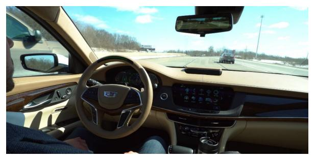
Cadillac's Super Cruise feature, seen here in the CT6, utilizes a driver attention system and LiDAR map data. These systems are added to the network of cameras and radar sensors already in the CT6. Super Cruise can automatically steer, brake, and keep the vehicle positioned on the highway in certain, optimal conditions. Photo: Cadillac.
