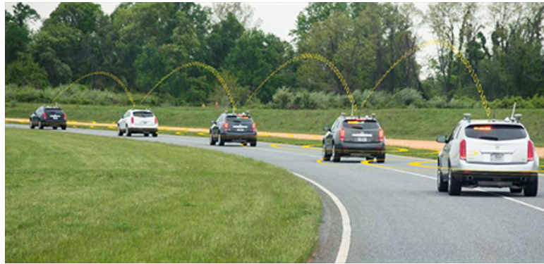
A group of self-driving cars successfully formed a platoon during a recent field test at Aberdeen Proving Ground, a U.S. Army test facility in Maryland. (FHWA photo)
