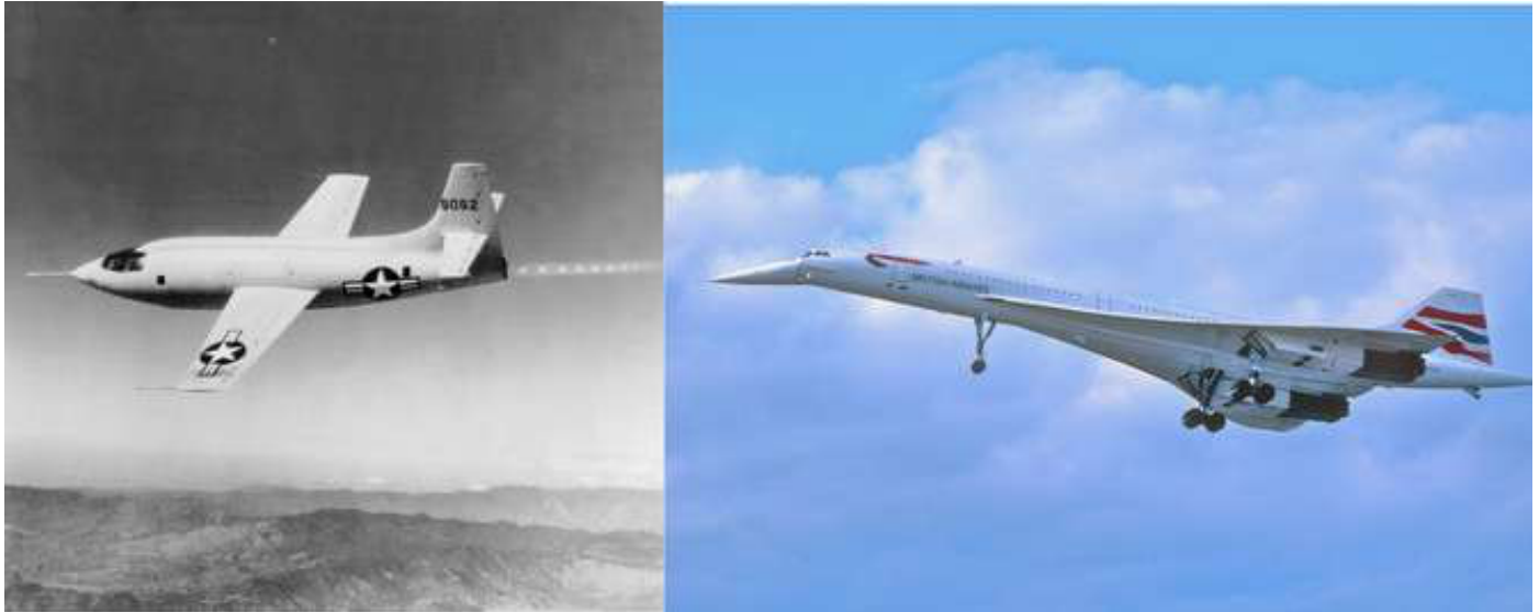
Left: the Bell X-1, the first supersonic aircraft. Right: a British Airways Concorde jet, the only commercial supersonic plane. Credit: Left: US Air Force. Right: Aero Icarus via Wikimedia Commons
