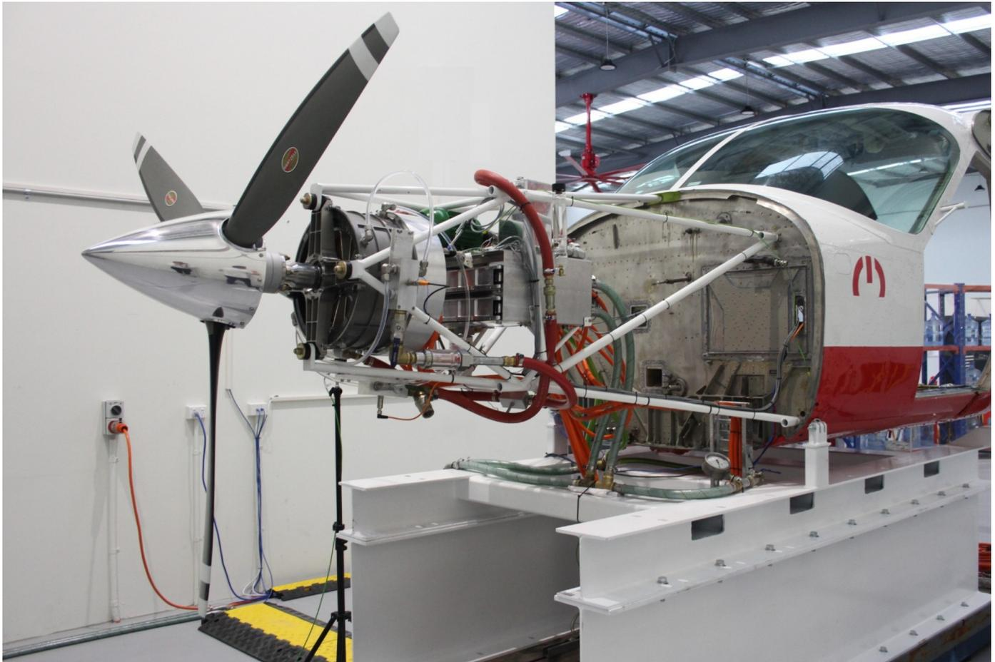
*Australian company Magnix is developing the electric engines for the Alice plane*
