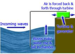
At a wave power station, the waves arriving cause the water in the chamber to rise and fall, which means that air is forced in and out of the hole in the top of the chamber.
