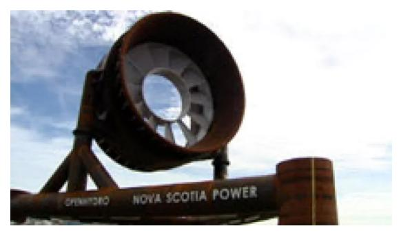
OpenHydro says the cause of the damaged test turbine in the Bay of Fundy was because of 10-knot currents, not ice as was One of the companies behind a large experimental tidal test project told a tidal energy conference Friday that powerful currents in the Bay of Fundy destroyed the blades of its <u>test</u> <u>turbine</u> in less than three weeks.
