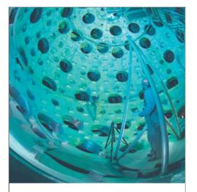
Laser-activated fusionInterior of the U.S. Department of Energy's National Ignition Facility (NIF), located at Lawrence Livermore National Laboratory, Livermore, California. The NIF target chamber uses a high-energy laser to heat fusion fuel to temperatures sufficient for thermonuclear ignition. The facility is used for basic science, fusion energy research, and nuclear weapons
