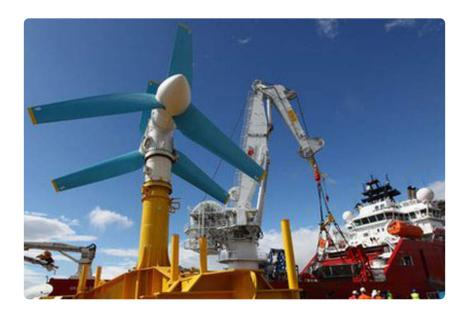
Atlantis Resources' AR1000 single-rotor tidal turbines are planned to be installed at the site. Image courtesy of Atlantis Resources Limited.
