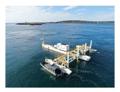
The combined project is to be called the Pempa'q In-stream Tidal Energy Project and will be delivered in phases starting next year. For Phase 1 SME will deliver three next generation PLAT-I platforms, each producing up to 420kW, providing a combined capacity of 1.26MW.
