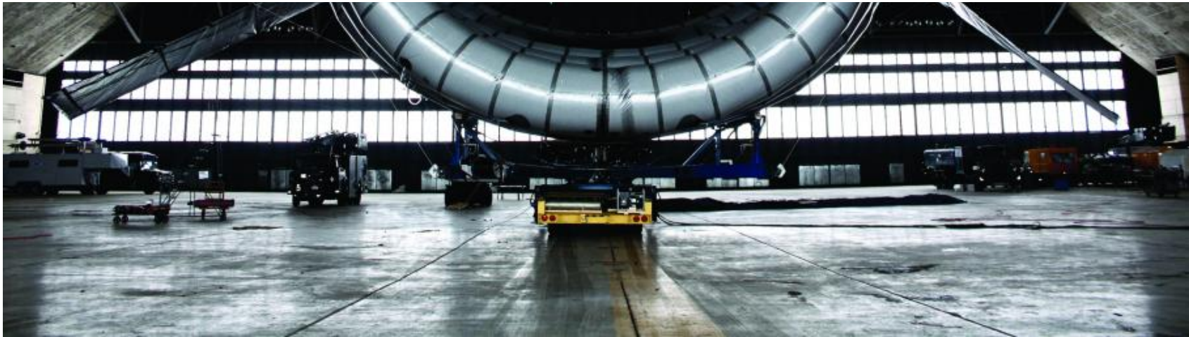
Altaeros' Buoyant Air Turbine Last year, Altaeros tested a prototype of the turbine at a height of 500 feet in Maine, where it flew in 45mph winds. courtesy Altaeros
