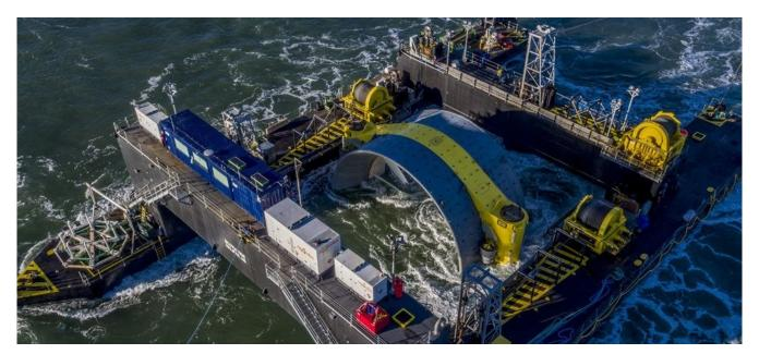
Cape Sharp Tidal's two-megawatt turbine is producing Canada's first in-stream tidal energy at the Fundy Ocean Research Center for Energy (FORCE) test site near Parrsboro, N.S. in November, 2016. Photo from CNW Group/Cape Sharp Tidal
