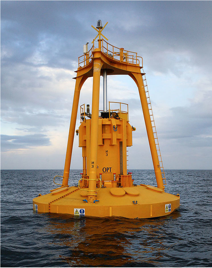
A major wave power installation off Australia's coast will use this type of power-generating buoy. OCEAN POWER TECHNOLOGIES, INC.
