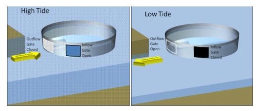
So a tidal lagoon is basically just a barrage that creates a circular pool within the larger area of the estuary rather than closing off the entire area with a dam the way a standard barrage does.
