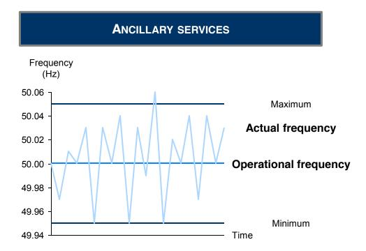
The system's frequency and voltage need to be maintained within technical limits to avoid instability and blackouts. This could be achieved by using fast-response electricity storage to inject or withdraw power as an alternative to conventional reserves(frequency response, spinning and non spinning, and replacement reserves).
