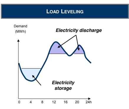
Electricity storage is used to level the load over various timescales. Typically, electricity is stored during periods of low demand and discharged during periods of peak demand to reduce the peak/off peak amplitude (daily, weekly and seasonal demand). This can also occur over shorter timescales (hourly) to smooth the load and avoid activating peak plants.
