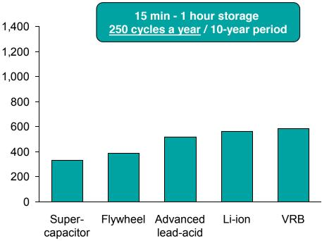
Technologies that benefit from a relative long cycling life (*e.g.* supercapacitors, flywheels) are favored over batteries for applications that require a high number of cycles (no replacement costs incurred over the 10-year period). High power capacity technologies (*e.g.* pumped hydro storage, compressed air energy storage) are not suited to short storage duration
