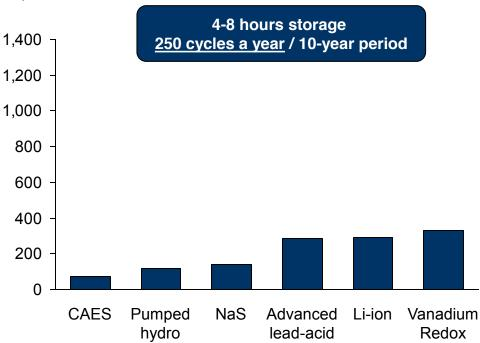
Compressed air energy storage is the most cost-effective technology for frequent discharging (1 cycle every day for 250 days per year) over long durations (8 hours) such as is required by power fleet optimization applications or price arbitrage (store during the night and discharge during the day).
